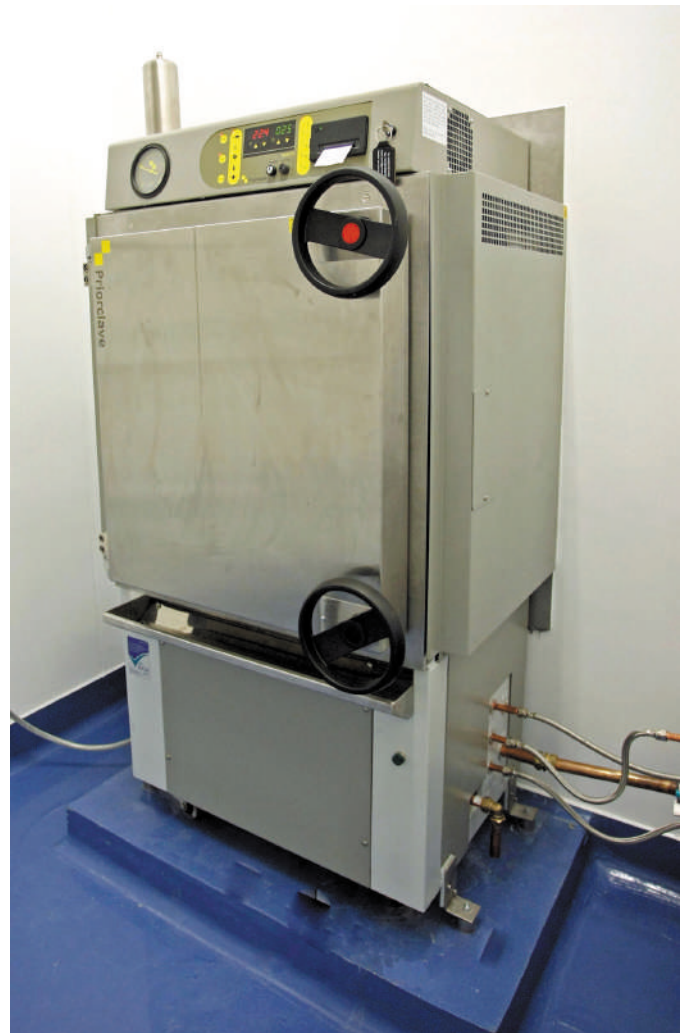
The service end showing the effluent retention filter protruding from the top and the TACTROL® data print-out record on the right of the fascia panel.
